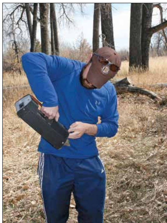
Figure 16. Crew member Dylan Mollendorf using the Mercury Vapor Analyzer in the ex situ method.
